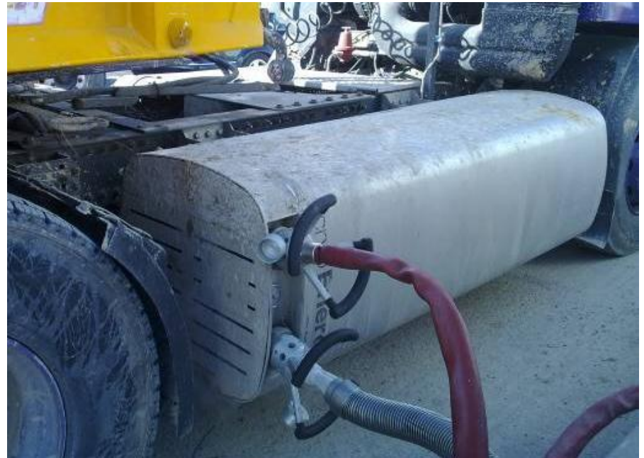
Double hose for filling and venting, high working pressure, 18 bar ( Indox ) (MB to adopt to 7-10 bar shortly)
